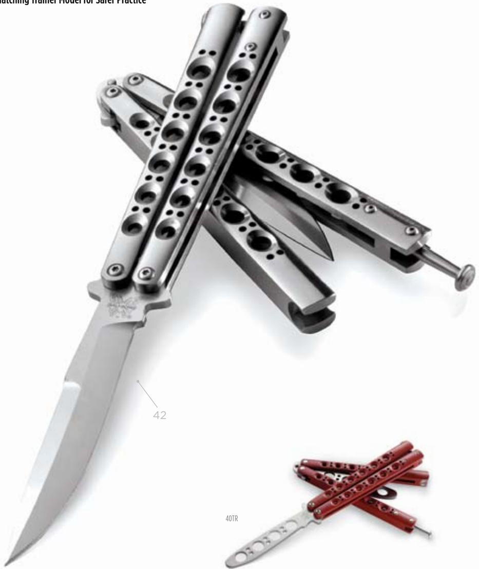
**42** DESIGNER: Benchmade LOCKING MECHANISM: Integrated Spring Latch BLADE STYLE: Weehawk BLADE STEEL: 154CM Stainless Steel (58-61HRC) BLADE LENGTH: 4.20" (10.67cm) BLADE THICKNESS: 0.125" (3.18mm) OPEN: 9.40" (23.88cm) CLOSED: 5.54" (14.07cm) WEIGHT: 4.40oz (124.74gm) HANDLE SPECS: Skeletonized Cast 6AL-4V Titanium HANDLE THICKNESS: 0.53" (1.35cm) SHEATH: Soft; Belt Carry COUNTRY OF ORIGIN: USA BLADE CONFIGURATIONS: 42 \$230
