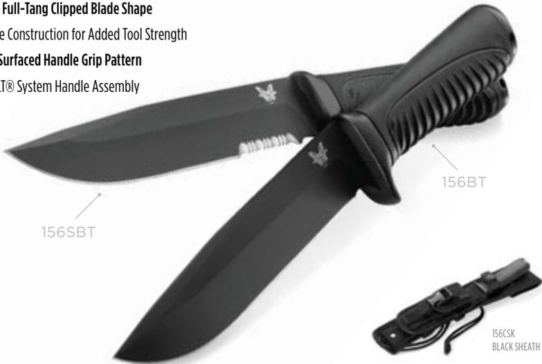
**156DESIGNER:** Benchmade **BLADE STYLE:** Combat/Survival Bowie **BLADE STEEL:** D2 Tool Steel (60-62HRC), BT Coated **BLADE LENGTH:** 6.10" (15.50cm) **BLADE THICKNESS:** 0.175" (4.45mm) **WEIGHT:** 9.60oz (272.16gm) **HANDLE SPECS:** Black Kraton® Overlay with BILT® System **HANDLE THICKNESS:** 0.78" (1.97cm) **SHEATH:** Multi-Function Soft Sheath, Removable Pouch, Black Nylon **SHEATH WEIGHT:** 6.50oz (184.27gm) **OVERALL LENGTH:** 10.90" (27.69cm) **COUNTRY OF ORIGIN:** USA
