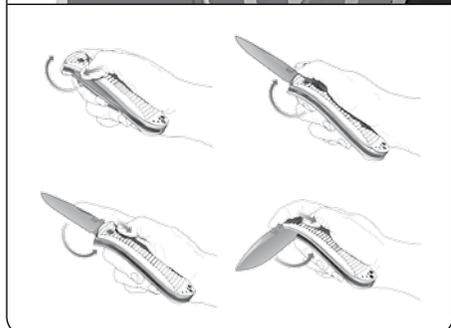
A patented Benchmade exclusive, AXIS has been turning heads and winning fans ever since its introduction. A 100-percent ambidextrous design, AXIS gets its function from a small, hardened steel bar which rides forward and back in a slot machined into both steel liners. The bar extends to both sides of the knife, spanning the liners and positioned over the rear of the blade. It engages a ramped, tang portion of the knife blade
