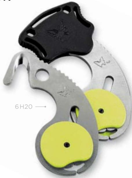
**6H20 DESIGNER:** Benchmade **BLADE STEEL:** X15 T.N Stainless Steel (58-60HRC) **BLADE OPENING:** 0.50" (1.27cm) **BLADE THICKNESS:** 0.115" (2.92mm) **WEIGHT:** 2.30oz (65gm) **HANDLE SPECS:** 6H20 Steel w/ Yellow Kydex Overlay **HARD SHEATH:** Molded Delrin Snap-Fit (Varied Carry Options Available) **HARD SHEATH WEIGHT:** 0.36oz (10.21gm) **OVERALL LENGTH:** 4.25" (10.80cm) **COUNTRY OF ORIGIN:** USA **BLADE CONFIGURATIONS:** **6H20** (Includes Hard Sheath) \$53
