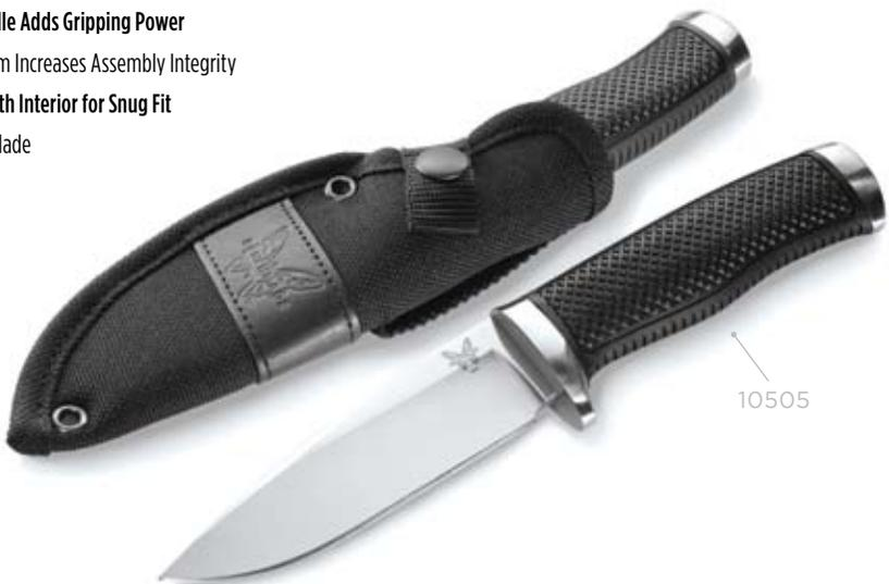
**10505 DESIGNER:** Mel Pardue **BLADE STYLE:** Drop-Point **BLADE STEEL:** 440C Stainless Steel (58-60HRC) **BLADE LENGTH:** 4.48" (11.38cm) **BLADE THICKNESS:** 0.139" (3.53mm) **WEIGHT:** 6.40oz (181.44gm) **HANDLE SPECS:** Polypropylene w/ Black Kraton® Overmold; w/ BILT® System **HANDLE THICKNESS:** 0.88" (2.23cm) **SHEATH:** Black Ballistics Nylon w/ Belt Loop **OVERALL LENGTH:** 9.11" (23.14cm) **COUNTRY OF ORIGIN:** Taiwan **BLADE CONFIGURATIONS:** 10505 \$65
