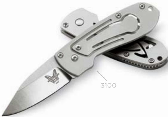
**3100DESIGNERS:** Bill McHenry & Jason Williams **LOCKING MECHANISM:** Auto-Levigator Lock **BLADE STYLE & OPENER:** Clip-Point, Auto-Levigator **BLADE STEEL:** 154CM Stainless Steel Hardened to 58-61HRC **BLADE LENGTH:** 1.95" (4.95cm) **BLADE THICKNESS:** 0.084" (2.13mm) **OPEN:** 4.75" (12.07cm) **CLOSED:** 2.84" (7.24cm) **WEIGHT:** 1.20oz (34gm) **HANDLE SPECS:** Stainless Steel **HANDLE THICKNESS:** 0.24" (0.61cm) **COUNTRY OF ORIGIN:** USA **BLADE CONFIGURATIONS:** 3100 \$125
