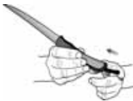
Push in tail-lock to lock blade
